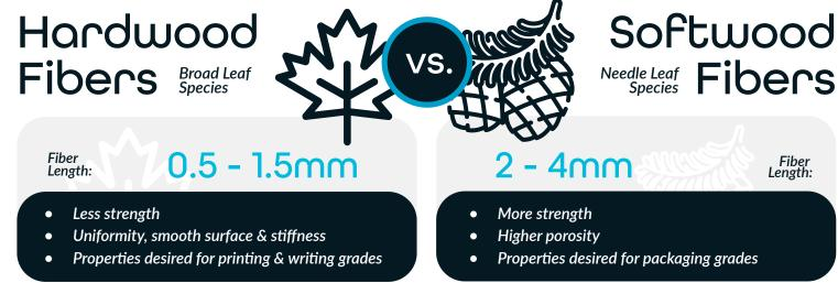
Based on paper grade requirements, it is fairly common to blend hardwood and softwood fibers to achieve the desired paper properties. Recipes can also be created to incorporate alternative fibers like bamboo and bagasse. The challenges associated with alternative fiber incorporation into wood fiber blends or existing equipment depends on the alternative fiber being used.
