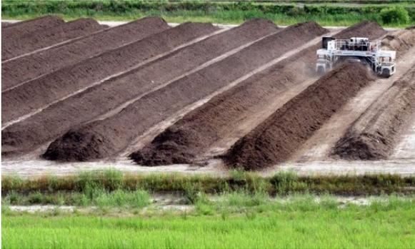
**Windrow composting**, in which organic waste is formed into rows of long piles and periodically turned, either manually or mechanically.
