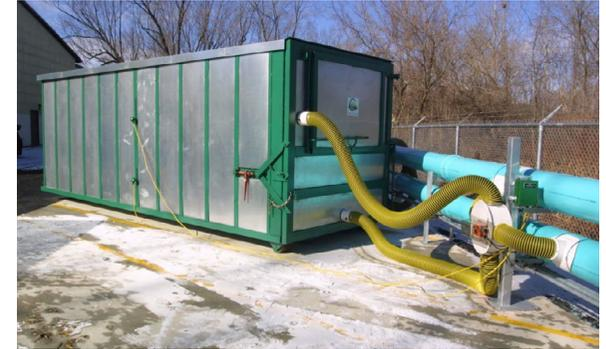
**In-vessel composting**, in which organic waste is fed into a drum, silo, concrete-lined trench, or similar equipment ([EPA](#)).
