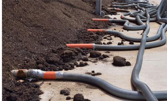
**Aerated static pile (ASP) composting**, in which organic waste is mixed in a large pile and designed so that air can pass from the bottom to the top of the pile. Piles are often aerated with a network of pipes, or with air blowers that are activated by a timer or sensor.
